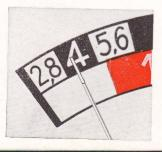
Adjust F/4 on the moving scale opposite the film group letter B, and read the F/ value i.e., f/2.8 on the moving scale by the side of 16 and set the lens accordingly.
