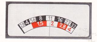
a) The deviation of the needle is read from the black upper scale.
