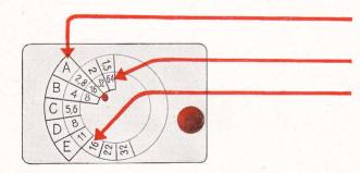
The letters A to E indicate groups under which headings the present day films have been listed (see group table). The operating speeds, 8 and 16 pictures a second etc. are read on the inner fixed scale. The F/ values are read from the instrument.
